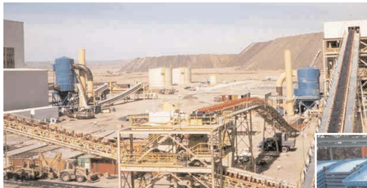
Two 1064AC12 filtering gold ore dust.
